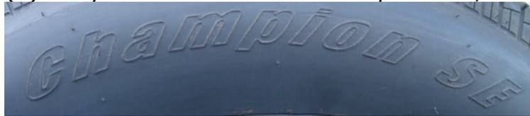
(2) The following information is molded into the sidewall of the tire below the "Champion SE" marking near the rim: "P235/75R15 105S". If any other size, such as P20575R15 is marked on the sidewall, your tire is not included in this recall.
